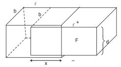
(ii) When battery is not connected  $F = \frac{Q^2}{2C^2} \frac{dC}{dx}$
